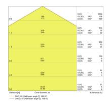
E(0") E(C90) 60.1° E(C0) 58.7° 2075 129 146 1.74 E(0°) E(C90) E(C0) 519 32 3.48 60.1° 58.7° E(0\*) E(C90) 60.1\* E(C0) 58.7° 231 14 5.22 4.93 E(0°) E(C90) 60.1° E(C0) 58.7° 6.96 6.58 E(0\*) E(C90) 60.1° E(C0) 58.7° 8.70 E(0°) E(C90) 60.1° F(C0) 58.7° 10.43 9.87 Cone diameter Im C0/C180 (Half beam angle [\*]: 117.4\*) C90/C270 (Half beam angle [\*]: 120.2\*)
