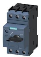
Circuit breaker size S0 for motor protection, CLASS 10 A-release 18...25 A N-release 325 A Screw terminal Standard switching capacity
