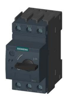
CIRCUIT-BREAKER SZ S00, FOR MOTOR PROTECTION, CLASS 10, A-REL. 0.55...0.8A, N-RELEASE10 A SCREW CONNECTION, STANDARD SW. CAPACITY
