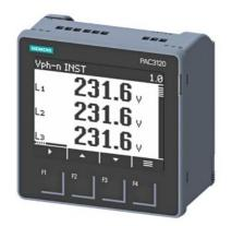
SENTRON PAC3120 LCD 96X96 mm Power Monitoring Device Controll panel instrument for electrical values protocol: Modbus RTU with graphics display U rated input: 690/400V 45-65Hz IE rated input: X/1A oder X/5A AC Power supply: 24 ... 60 V -20/+10 % DC screw connections
