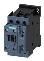
Power contactor, AC-3 32 A, 15 kW / 400 V 1 NO + 1 NC, 230 V AC 50/60 Hz, 3-pole size S0 screw terminals
