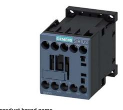
Power contactor, AC-3 16 A, 7.5 kW / 400 V 1 NO, 230 V AC, 50/60 Hz 3-pole, Size S00 screw terminals
