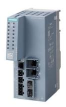
SCALANCE SC632-2C Industrial Security Appliance; For protection of devices and networks in discrete manufacturing and the process industry For protection of industrial communication with firewall; Further functions: Address translation (NAT/NAPT); Connection to SINEMA RC; 2x combo port electrical or optical; 10/100/1000 Mbps RJ45 or 100 Mbps SFP or 1000 Mbps SFP
