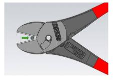
First make a notch in the wire using the KNIPEX TwinForce until the required hand force increases considerably. Now open the pliers and slide the wire backwards towards the joint. Hold the cutting edge in the notches you have made in step 1.
