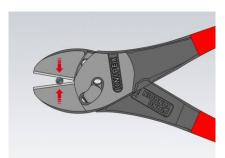
Insert the wires as close to the hinge as possible. In case of cutters with very high transmission, the width of the gap between the cutting edges close to the fulcrum may be less than the thickness of the wire. Wires may slip forward when the cutting starts.
